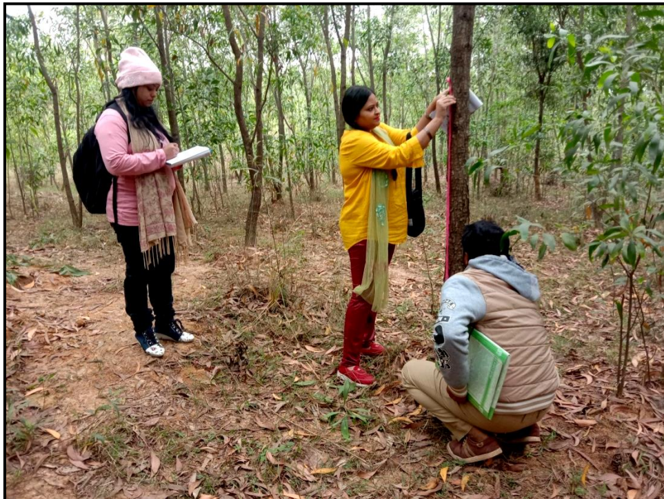
Fig. A8: Measuring the DBH at 1.37 meter height from the ground
